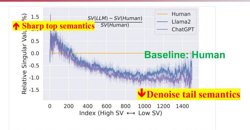
Figure 7: Comparision of the relative singular value (SV) of the different corpus after SVD. The singular values are sorted in descending order from left to right.
